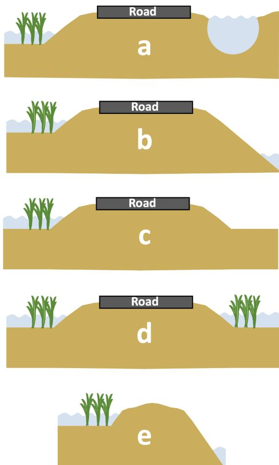
Fig. 2. Cross-section diagrams of common levees in California rice fields, separated based on the features they border. These include levees with unpaved access roads bordering a) supply canals, b) drainage ditches, c) fallow fields, and d) flooded fields with a higher or lower relative water height. Some levees also bordered a drainage ditch but were narrower with no access road (e).
